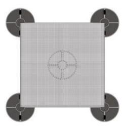
SIZE 40X120 cm: 1 support for each corner, 2 supports 1/3 along the slab and 2 supports half-way along each of the two long sides (4 supports per piece)
